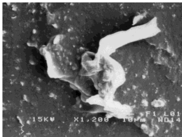
Figure 5 Ribbonlike wear debris on 1% LC2 PA 6 (steel pin; 80°C).
